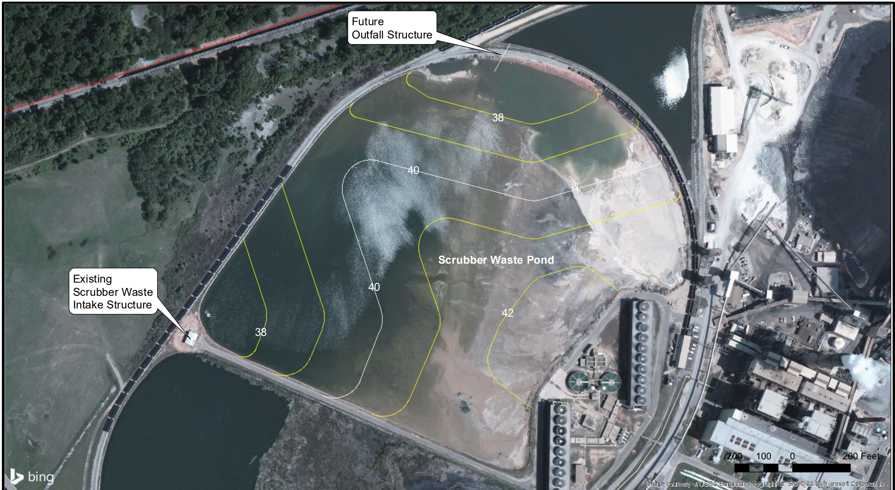
Figure 3 -Scrubber Waste Pond Final Grading and Stormwater Control Plan Charles R. Lowman Power Plant Leroy, AL
